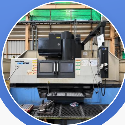
DOOSAN VM750 1800x750x800mm RPM 12,000 Pull stud 50° BT 50
