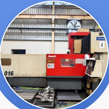
AWEA SP3016 3000x1600x1000mm RPM 10,000 Pull stud 60° BT 50
